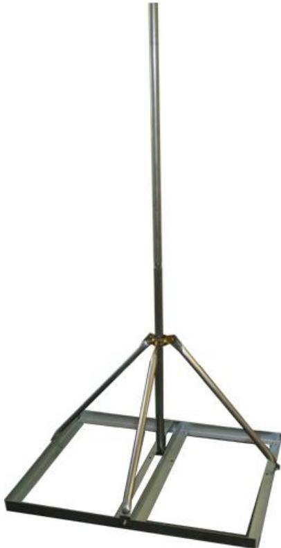
Avoid drilling lag screws into your flat roof top or concrete pad, the EZ-NPP is recommended for high wind installations, providing a strong platform with cinder blocks for ballast (cinder blocks are not included).
